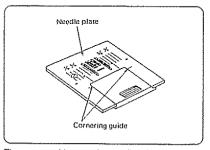
The seam guides on the needle plate help you measure seam width. The lines are 1/8" apart, with the 5/8" and 7/8" lines marked.
